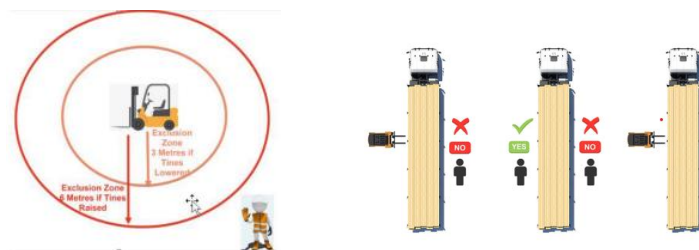
Figure 3 Exclusion Zones – Single and Multiple Adjacent Bays
