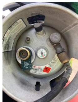
Figure 4 Pressure relief valve is at 12 o'clock when cylinder is oriented correctly.
