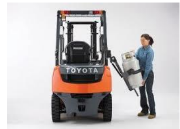
Figure 5 LPG cylinder bracket is adjustable on this plant to bring down to between waist and shoulder height for removal.
